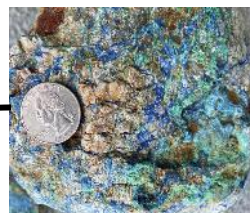
Azurite-malachite-chrysocolla in oxidized quartz vein with limonite and late azurite veinlets
